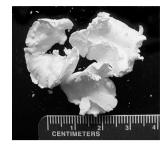
From a facile catalyst-free method, pure single-crystalline nanotetrapod-assembled ZnO was grown on a gram-scale for the first time, with high repeatability and conversion efficiency. All four arms of the nanotetrapods are cone shaped and grow in the [001] direction. The photoluminescence properties were studied and a mechanism was suggested for the growth of the nanotetrapod-assembled ZnO.
